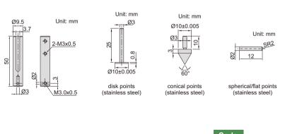
■ Suitable for 0-150mm/0-6" and 0-200mm/0-8" digital calipers (thickness of lower jaws≤3.7mm)
